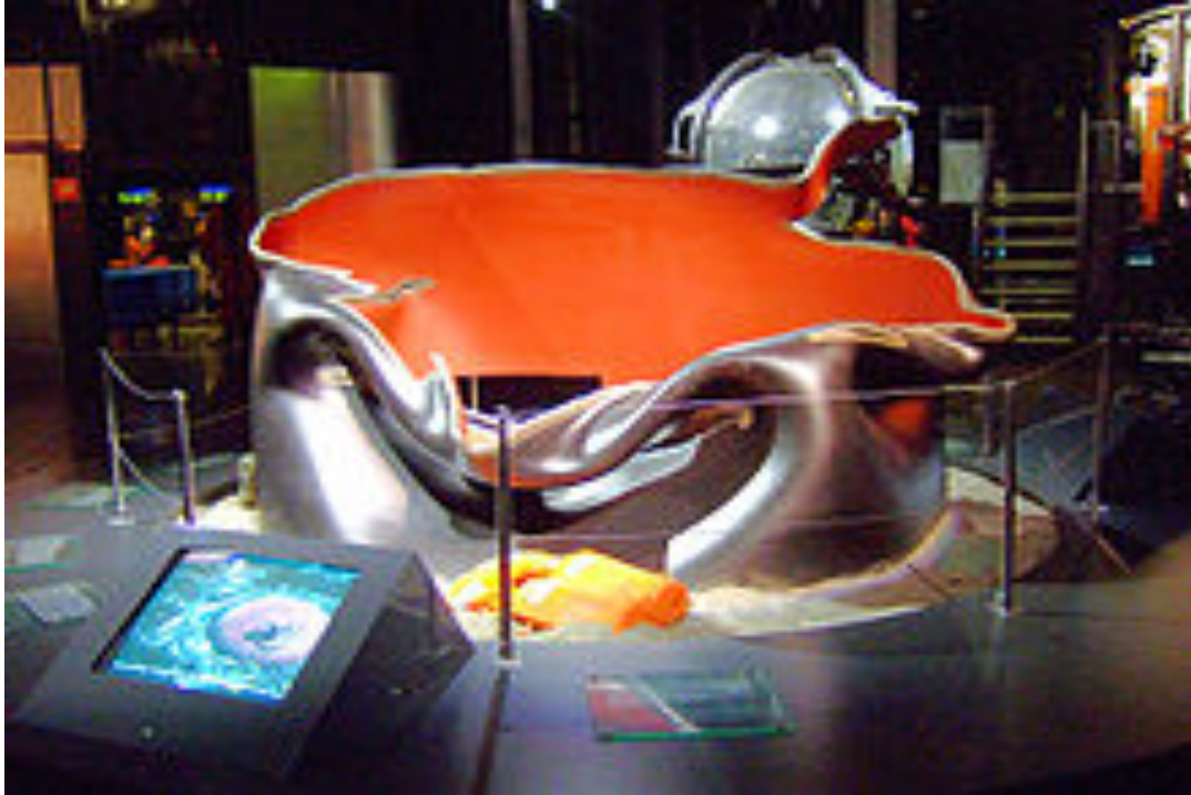
Figure 1 : How a tubular product form would look if it had been overloaded derived from incorrect stress design calculations and or operational abuse.
