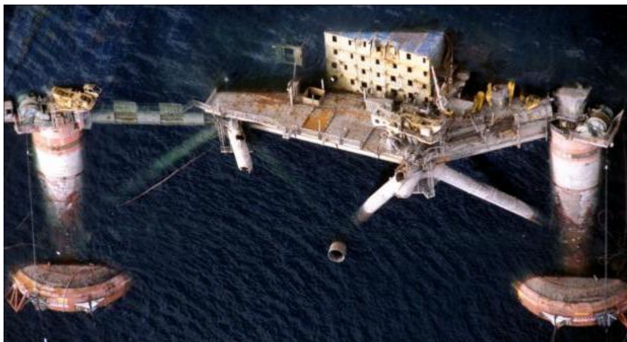
Figure 3 : Overall view of the collapsed platform/rig showing no evidence of plastic deformation in the component parts, therefore no evidence for abuse that would cause overload and collapse.
