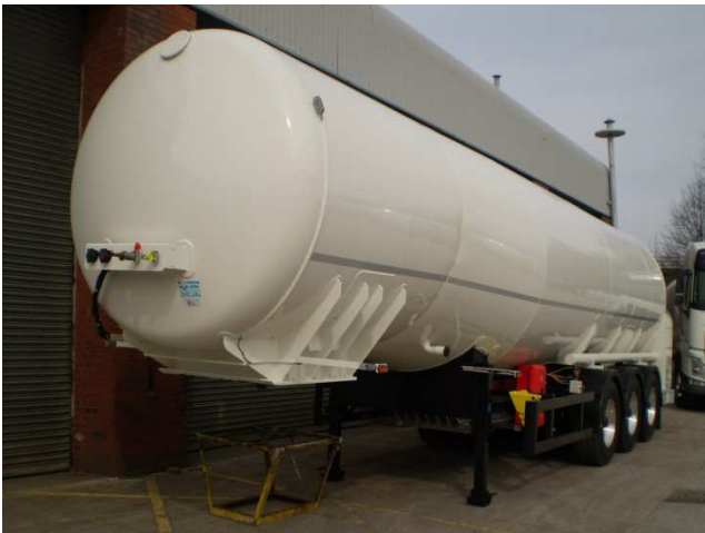
Figure 18. Road going liquid gas containing pressure vessel equipment demands high weld quality fabrication, i.e. welds with a controlled low level of imperfection in all aspects. This fabrication quality can and is achieved by implementing the established welding principles. Photograph courtesy of M1 Eng. Ltd, Bradford, UK.
