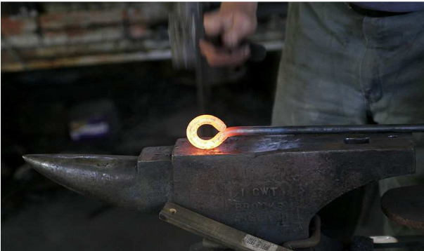
Figure 9. Blacksmith forge welding.
