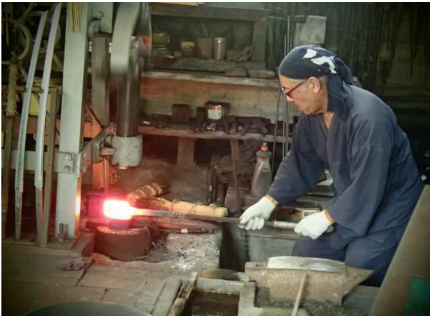
Figure 5. Japanese Samurai sword maker forge welding the blade.
