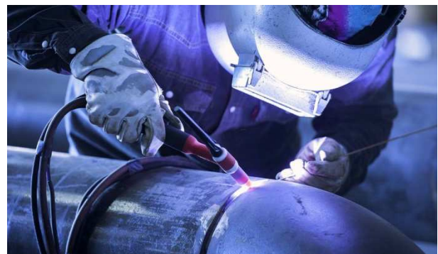
Figure 13. The Tungsten Inert Gas (GTAW) Process with ceramic, torch components and shield gas cup.
