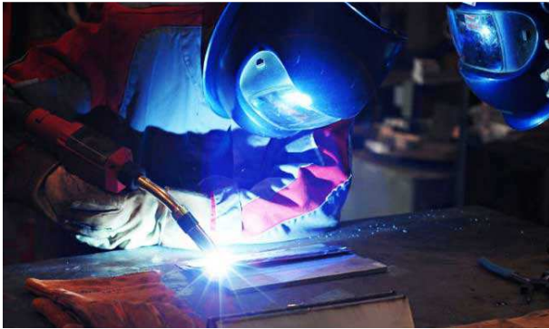
Figure 14. The Metal Inert/Metal Active Gas (GMAW) welding process.
