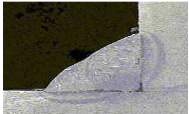
Figure 17. Physical imperfections in a fillet weld, lack of:- root fusion, sidewall fusion and penetration.
