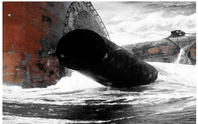
Figure 7. The collapsed Alexander L. Kielland Oil Platform showing the failed brace D6 and the true source of the propagated crack which was the hydrophone insert welded joint. No qualified, weld procedure, welder and inspection techniques were used to manufacture this welded joint, a catastrophic failure was incurred as a result of this behavior.
