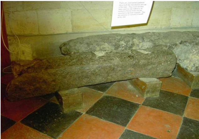
Figure 3. Roman hypocaust lintel over 1 metre long and weighing some 40 Kg fabricated by forge welding a number of smaller ‘blooms’ of Iron by repeated heating and hammering.
