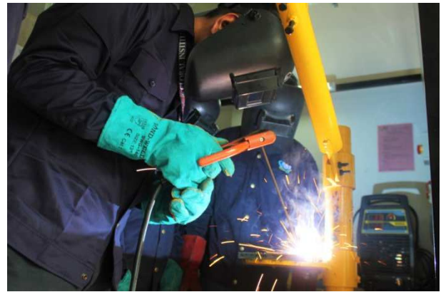
Figure 10. The Manual Metal Arc welding process with flux coated electrode, brought into production of the Liberty Ships during WWII.
