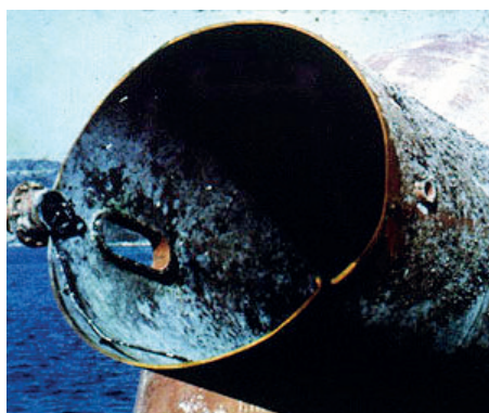
Fig 4. The John Thompson pressure vessel that failed upon hydraulic testing - 'Abandon the weld procedure at your peril'
