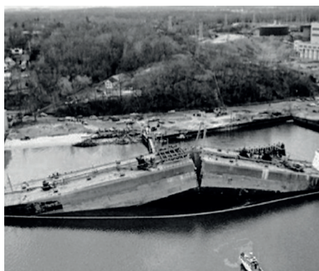
Fig 3. A WW II Liberty ship brittle fracture failure
